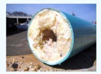
Above is the result of flushing fats, oils and grease. Sanitary sewer mains and residential/commercial laterals can become blocked and this will lead to many complications with public and residential/commercial systems.
